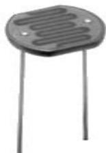
Typical LDR, As its name implies, the Light Dependent Resistor (LDR) is made from a piece of exposed semiconductor material such as cadmium sulphide that changes its electrical resistance from several thousand Ohms in the dark to only a few hundred Ohms when light falls upon it by creating hole-electron pairs in the material.
